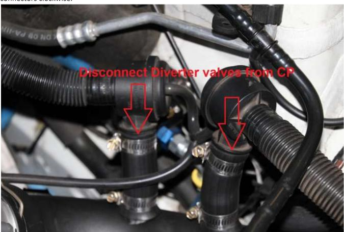
d. Disconnect the front intake diverter valve line.
