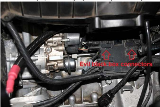
b. Sorry...bad picture. If you use a flat head screw driver to leverage against the tabs, you can push the metal tabs through the slots. The one on the left I use two screw drivers due to the distance.
