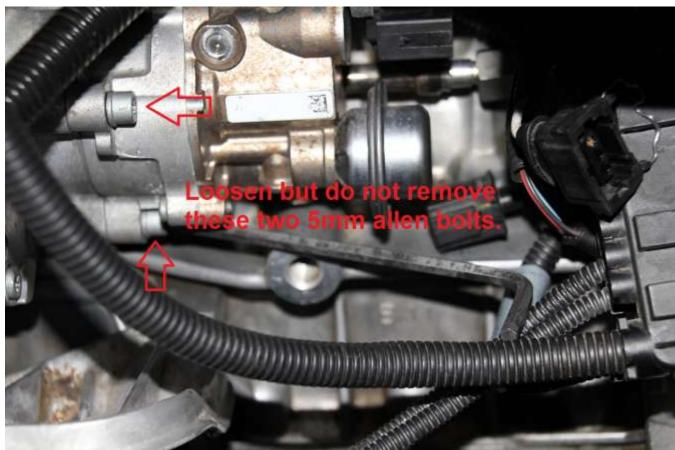
h. Now the hardest part...there is one 5mm allen bolt on the back side of the pump. In this picture you can see the locations of the bolts.
