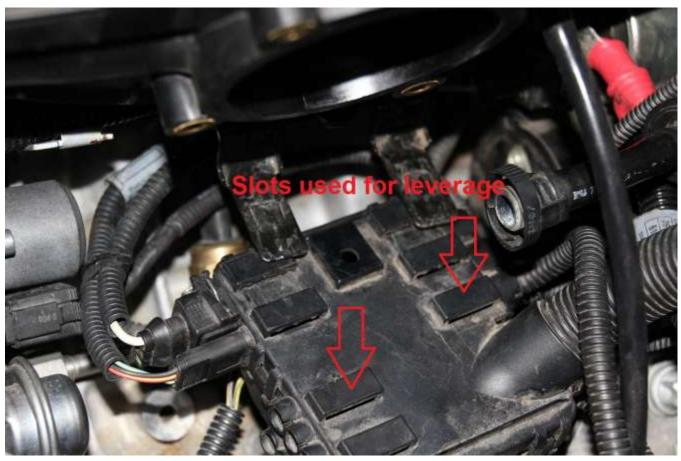
c. Disconnect the two electrical connections on the left side of the black box to move it further out of the way. (optional but easier)
