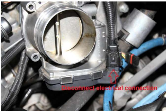
e. I use a small tweaker to lift the tab to disconnect it. (you won't have the Fuelab FPR on the right)
