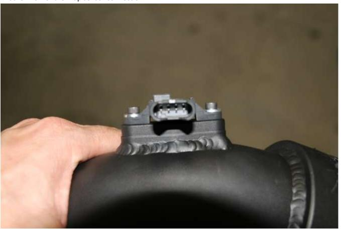
e. Remove the charge pipe (there is an o-ring inside...don't lose it and verify it's there)
