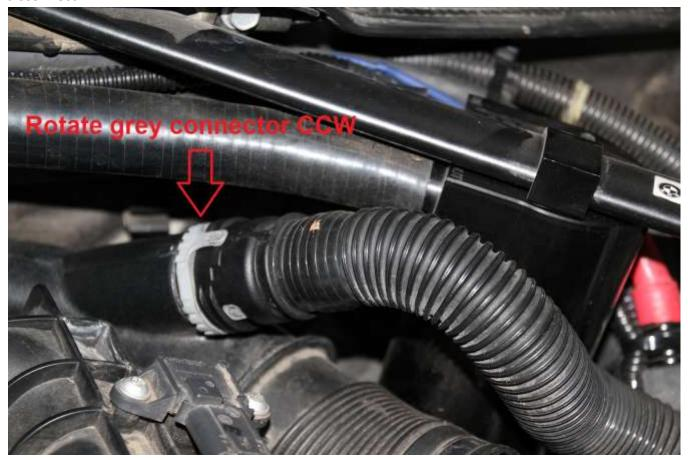
b. Disconnect the vacuum line at the Y connector (don't disconnect manifold side to prevent breakage).
