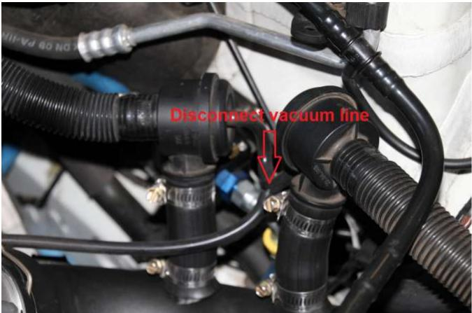
c. Disconnect the diverter valves from the charge pipe. If you have a stock CP, you will rotate the grey connectors clockwise.
