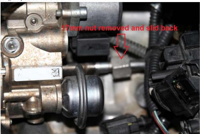
e. After the inlet line is disconnected, there should be enough flex and room to push the inlet line away from the HPFP and toward the block to disconnect it from the HPFP. If it's too tight, you can loosen the clamp near the LPFP sensor so the line can slide. Sorry didn't get the size of the torx nut.
